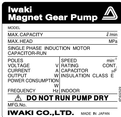
Spec label (pump unit) for any area other than the European market
